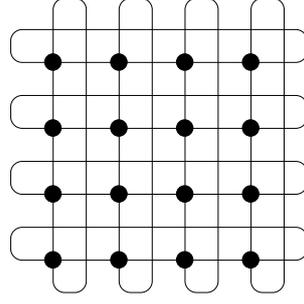
**Figure 2:** A  $4 \times 4$  Bidirectional Manhattan Network
