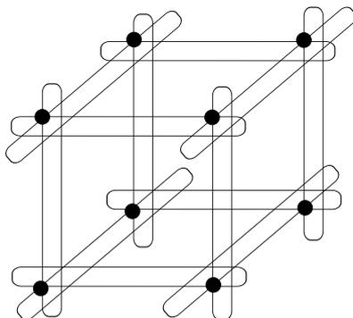
**Figure 3:** A 3-dimensional torus of dimension 2
