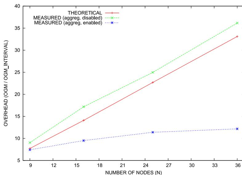
**Figure 5:** Number of OGM messages sent out by every node every *OGM\_INTERVAL* in a Manhattan topology. Are reported the expected values and the measured ones both with aggregation enabled and disabled.
